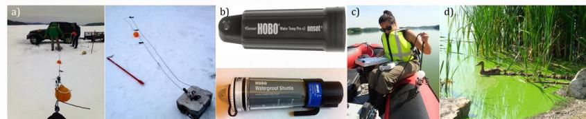
Figure 4. a) The thermistor chain is composed of five temperature HOBO® Water Temp Pro v2 u22-001 loggers and was installed when the pond was still frozen. b) HOBO® Water Temp Pro v2 u22-001 loggers (top), and HOBO® Waterproof Shuttle data downloader (bottom). c) Collecting Photosynthetically Active Radiation (PAR) measurements during weekly sampling. d) Cyanobacteria bloom on June 17, 2014.
