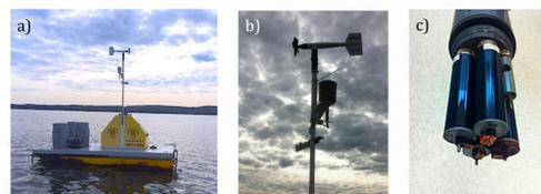
Figure 2. Buoy system on Missisquoi Bay (a) that contains automatic samplers for water, weather station (b) and YSI Sonde (c).
